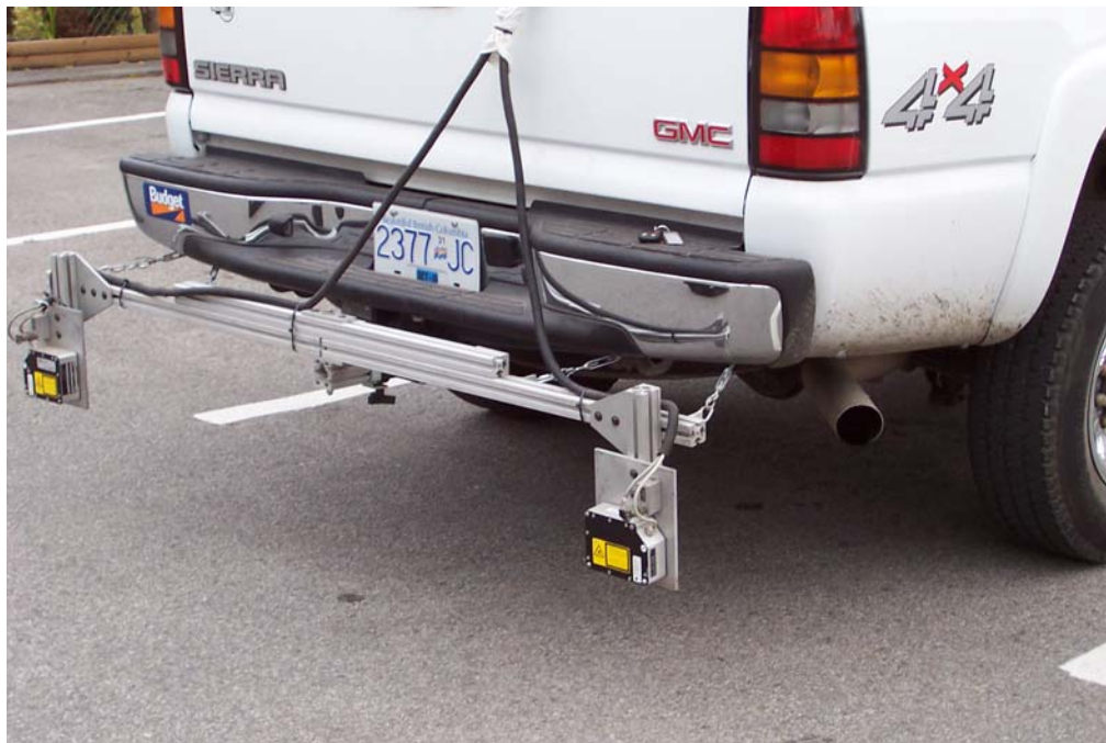
Figure 4. Bumper mounted laser profiler used for IRI measurement.
