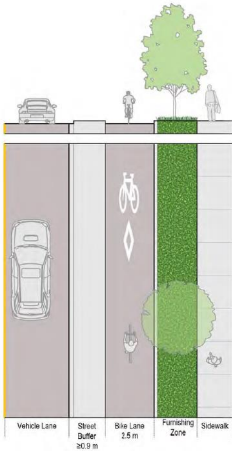
FIGURE D-38 // UNI-DIRECTIONAL PROTECTED BICYCLE LANE CROSS-SECTION - NO ON-STREET PARKING (DESIRED WIDTH)
