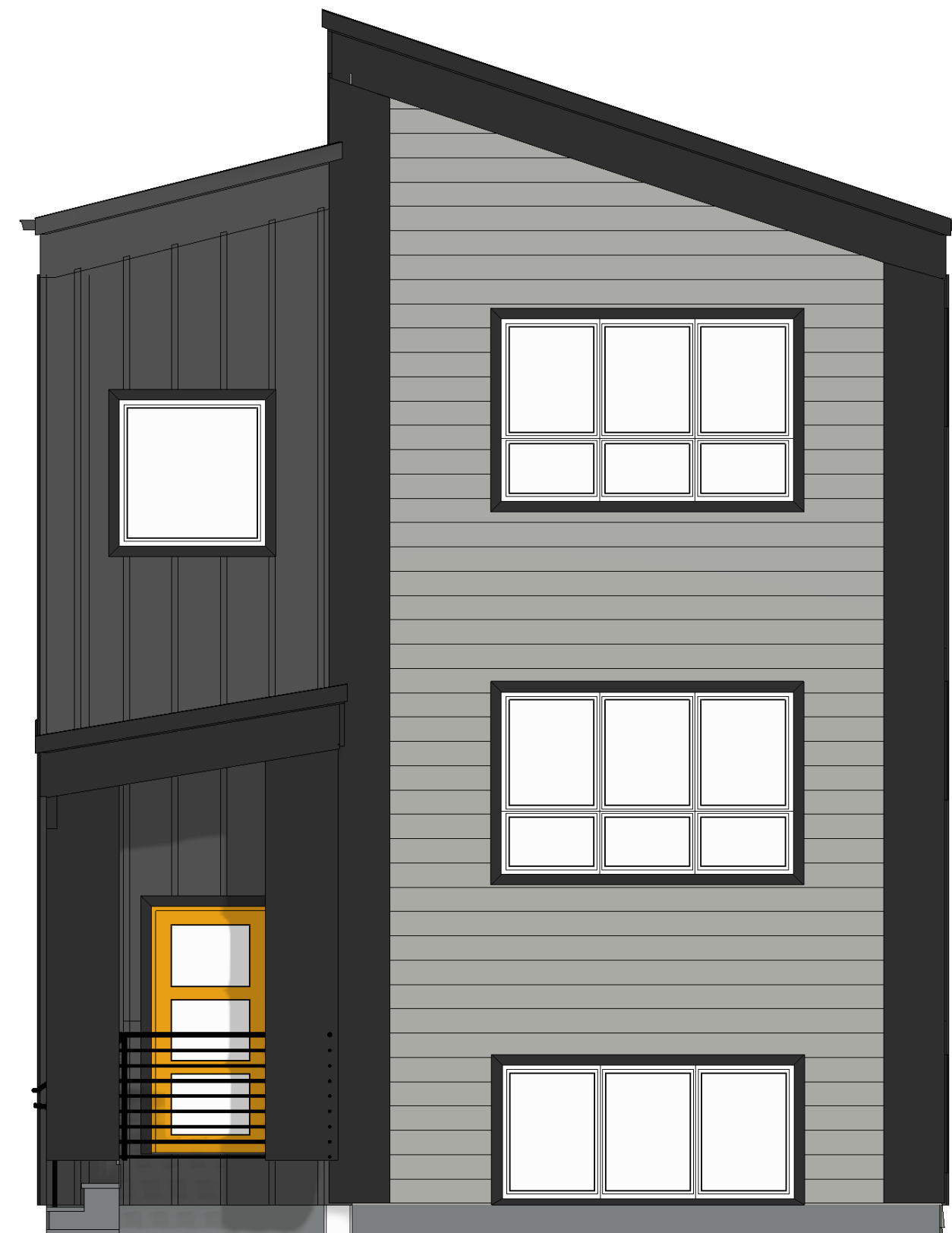
SOUTH ELEVATION (FACING LANE) SCALE: 1/4" = 1'-0"
