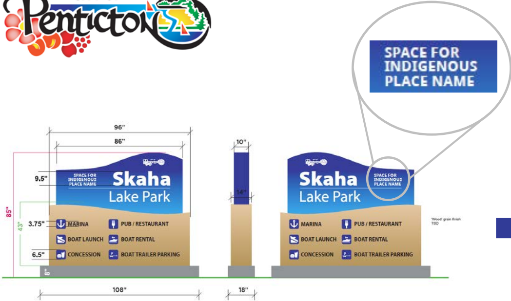
non-illuminated powder-coated aluminum monument sign with acrylic text and faux wood finish
